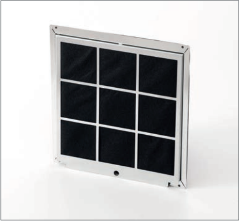
FILTRI A CASSETTA IN ALLUMINIO CASETTE CARBON FILTER Questi filtri devono essere lavati, o sostituiti, ogni 3-5 mesi. Possono essere lavati a mano o in lavastoviglie (temperatura max 55 °C)., fino ad un totale di cinque lavaggi. Per asciugare il filtro interno, esporre all'aria o inserire in forno a 80° max per 40 minuti. The service time in case of use of the cooking range is 3-5 month, afterwards, it has to be replaced or washed. Washing may either be performed by hand or in a dishwasher with regular programme of max. 55° C with a standard washing programme. For drying, either expose the filter pad to the air or dry in the oven at max. 80° C for 40 minutes. It should be replaced with a new one after maximum of 5 washes.
