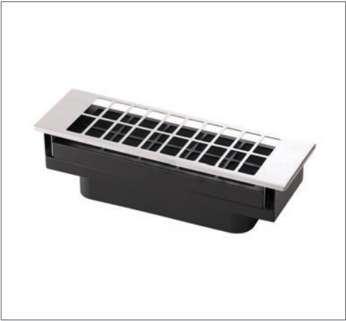
FILTRO CARBONE HELSEA HELSA CARBON FILTER Ogni 3-5 mesi sostituire o pulire in forno (ca 60-90 minuti a 175-200°C) The service time in case of use of the cooking range is 3-5 month, afterwards, it has to be replaced or cleaned in oven. (Approximately 60-90 min. At 175-200 ° C)
